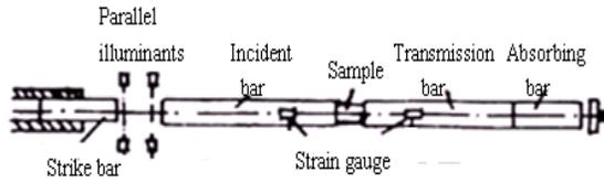
Fig. 1: Typical SHPB experimental device
