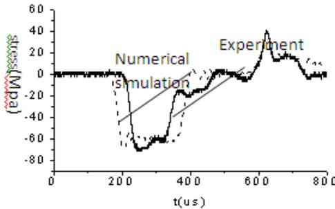
Fig. 9: The curves of incident wave and reflected wave
