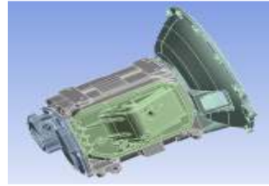
Fig. 1: 3D assembly model of the transmission housing and the clutch
