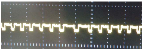
Fig. 13: Ignition drive signal when duty cycle 30 and speed 5300 r/min
