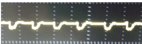
Fig. 14: Ignition drive signal when duty cycle 30 and speed 4300 r/min
