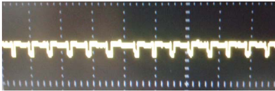
Fig. 12: Ignition drive signal when duty cycle 20 and speed 5300 r/min
