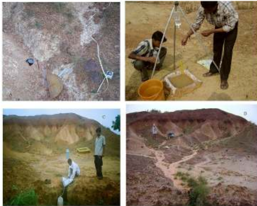
Fig. 2: (a) Monitoring junction angle and gradient of the merging links in field, (b) measurement of infiltration in field through a plot of 1×1 feet area with regulated supply of water for duration of 5 h. until a constant rate is reached following (Goudie, 1990), (c) collection of water and sediment discharge at the gully mouth during a rain, recorded by rain gauge. The infiltrated water was also collected simultaneously from the base of a representative plot (1 m × 1 m) set the field with an average gradient for comparison with the former. Only little variation is observed between these two methods, (d) Monitoring discharge by setting ‘V’ notch at each junction connected with the bottles for collection of entire flow of water and sediment; the rain input is recorded in the field with recording type rain gauge
