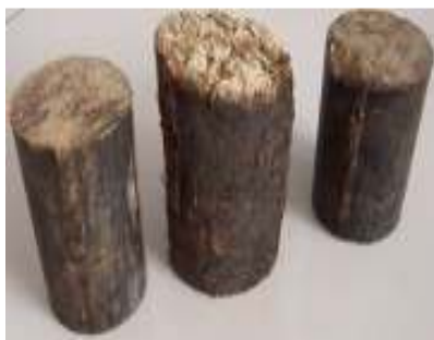
Fig. 2: Corn stover briquettes extruded from HPB-III briquetting machine
