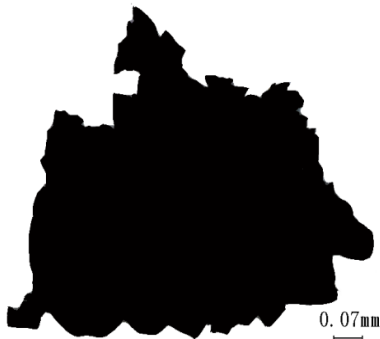
(b) Pore in un-cracked concrete
