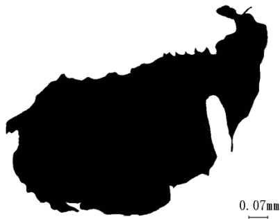
(a) Pore in cracked concrete
