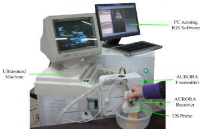
Fig. 3: Phantom experiment configuration
