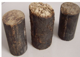
Fig. 2: Corn straw briquettes extruded from HPB-III briquetting machine
