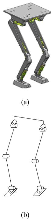
Fig. 1: The structure of the hydraulic biped robot: (a) mechanical structure, (b) DOFs distribution
