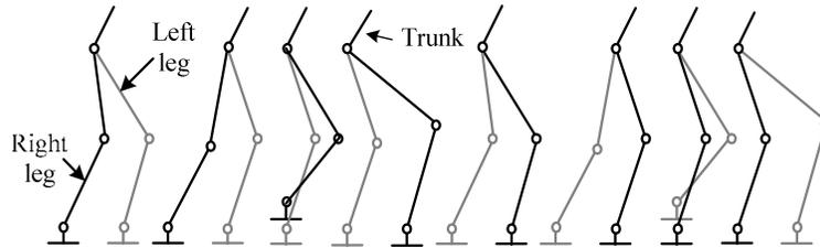
Fig. 4: Motion sequences of the biped robot with static walk
