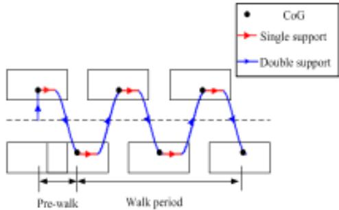
Fig. 7: The trajectory of CoG on ground while walking in the improved pattern
