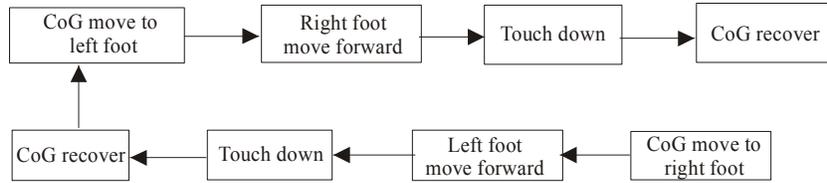
Fig. 3: The process of biped robot's static walk
