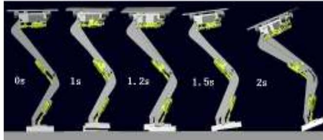
(a) The simulation of static walk: cycle time set to 2s, step length set to 80 mm, step height set to 30 mm
