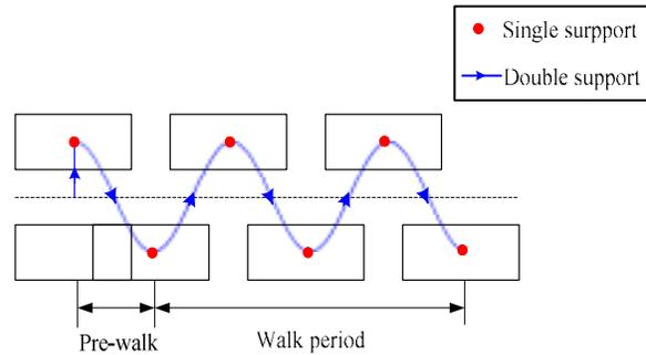
Fig. 5: The trajectory of CoG on ground while in static walk
