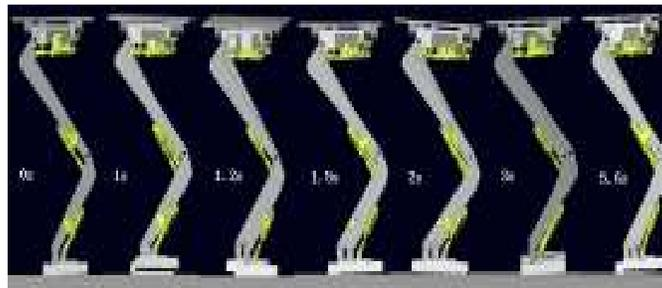
(b) The simulation of improved walk: cycle time set to 2s, step length set to 80 mm, step height set to 30 mm
