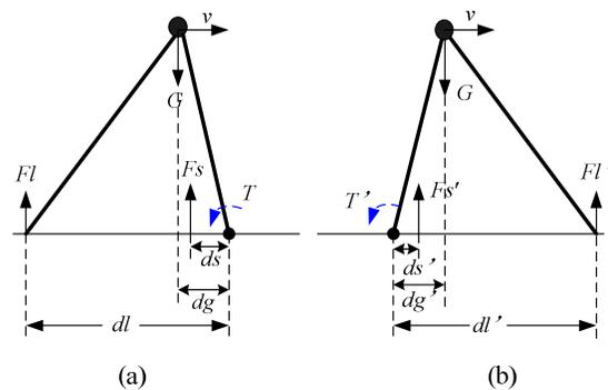
Fig. 6: An analysis about the biped robot while in static walk: (a) from double support phase to single support phase, (b) from single support phase to double support phase
