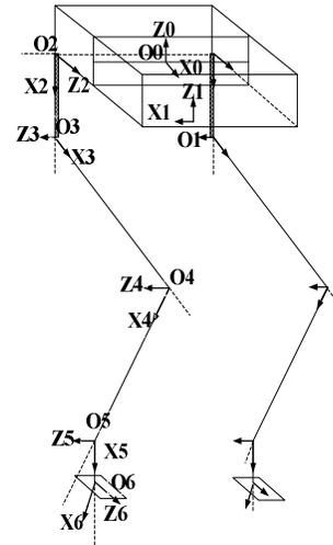
Fig. 2: Local frames linked to the biped robot
