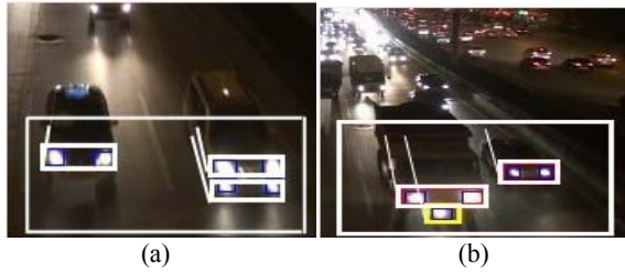
Fig. 5: Examples of redundant trackers (a) two trackers tracking a vehicle (b) two trackers tracking a truck
