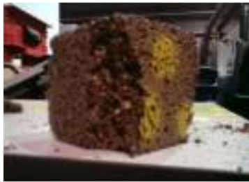
Fig. 7: Failure of concrete with 50% COPS
