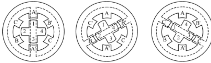
Fig. 1: Principle of 3-phase reactive stepping motor
