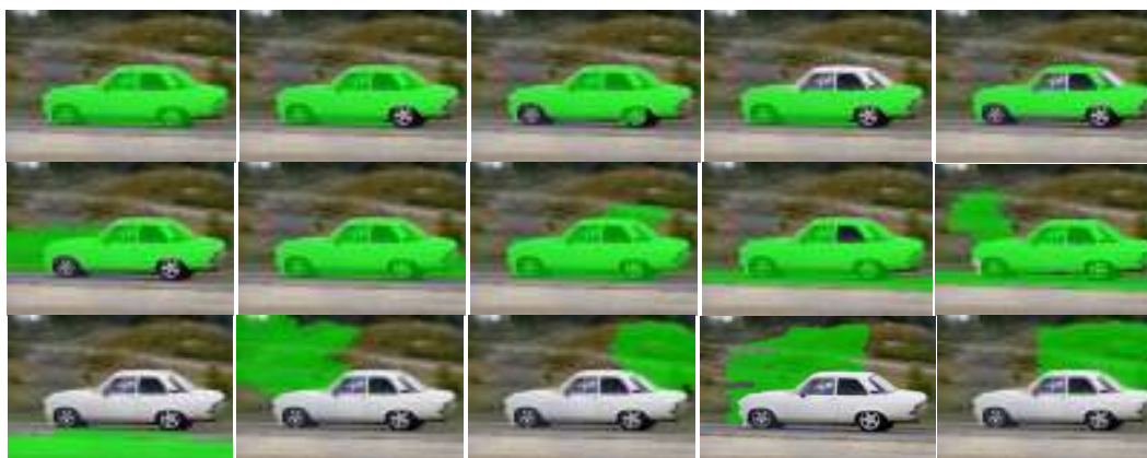
Fig. 2: Examples of segments generated by CPMC algorithm colored in green (best viewed in color)
