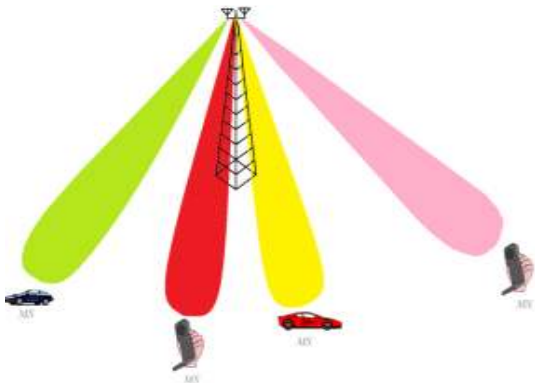
Fig. 3: Transmit Beam Forming depending on the angle of each user (Rank 1 CLSM)
