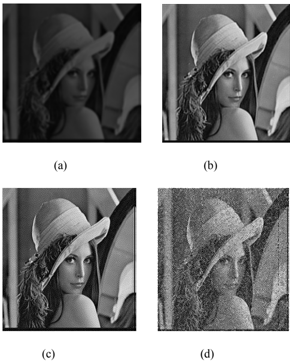
Fig.7: The restored image at different estimated SNR (a) when the estimated SNR is 20 dB (PSNR = 24.5809 dB), (b) when the estimated SNR is 45 dB (PSNR = 30.0017 dB), (c) when the estimated SNR is 60 dB (PSNR = 28.8848 dB), (d) when the estimated SNR is 80 dB (PSNR = 27.3557 dB)
