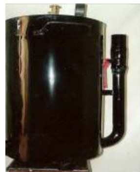
Fig. 1: Bioreactor used for production of biogas by anaerobic digestion of water hyacinth
