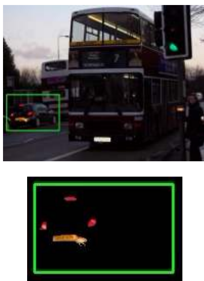
Fig. 3: A failed example of grab cut algorithm
