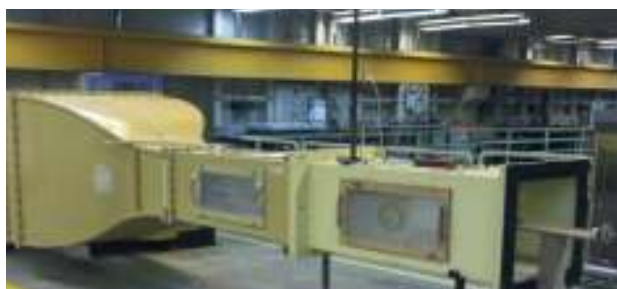
Sub scale model and plinth 600x600 mm subsonic wind tunnel
