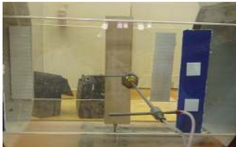
Fig. 2: Lift and drag measurement on 300 mm aerofoil model in Arms field 300x300 mm subsonic wind tunnel
