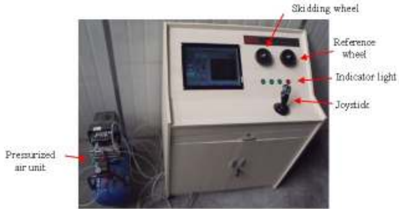
Fig. 4: The appearance of the semi-physical simulation platform
