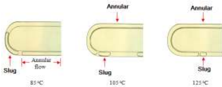
Fig. 3: Internal flow patterns of HHMCLOHP/CV using a ethanol at Le of 50 mm
