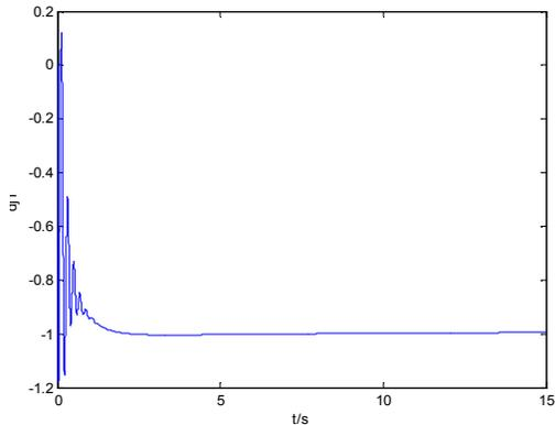
Fig. 12: Rudder response for sliding mode control
