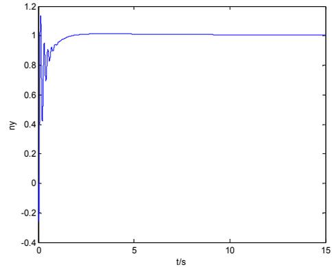
Fig. 9: Overload response for sliding mode control
