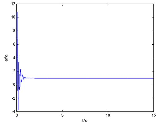
Fig. 11: Attack angle response for sliding mode control
