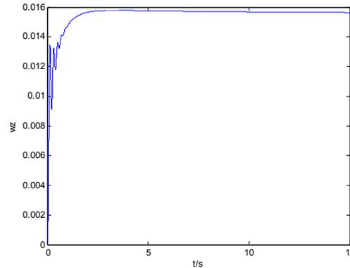
Fig. 10: Angle rate response for sliding mode control
