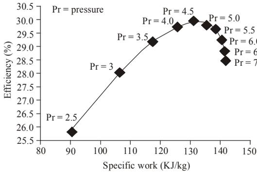
Fig. 2: Performance characteristic curve of microturbine
