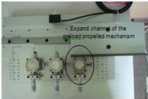
Fig. 11: The stereogram of a long distance piezoelectric actuated stage
