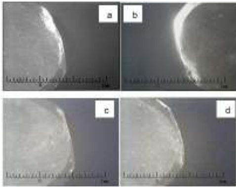
Fig. 2: Wear on CBN tool
