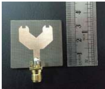
Fig. 2: Fabricated antenna element photograph
