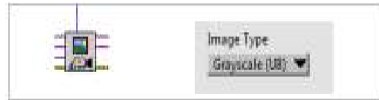
Fig. 10: Frame grabber block in Labview and image type setting
