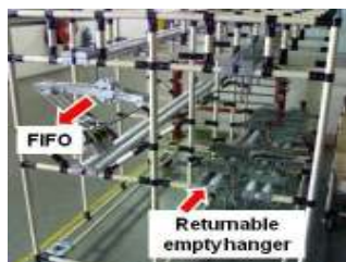
Fig. 5: The FIFO method in the minomi concept
