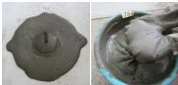
Fig. 7: Picture of slump on mass concentration 75%
