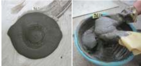
Fig. 6: Picture of slump on mass concentration 76%
