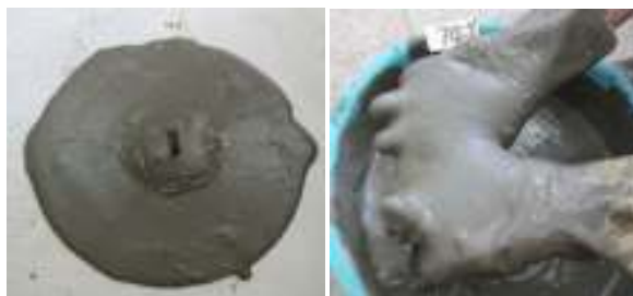
Fig. 8: Picture of slump on mass concentration 74%
