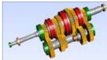
Fig. 8: 3D model view of the transmission (excluding housing)
