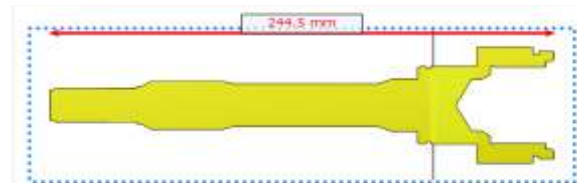
Fig. 2: The input shaft model of the manual transmission
