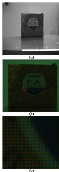
Fig. 1: (a) The Y800 original data of a box, (b) convert the Fig. 1a to a 24-bit image, (c) the enlargement of the small red box of Fig. 1b
