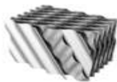
Fig. 1: A schematic view from the horizontal corrugated film packing type
