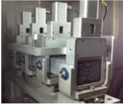
Fig. 2: Four-points bending fatigue test setup
