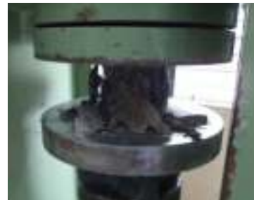
Fig. 4: Splitting failure of CPFRC in compression
