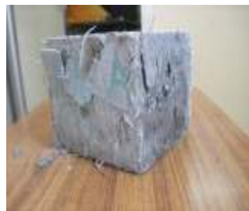
Fig. 6: Multiple cracking mode of CPFRC specimens after post peak load
