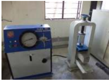
Fig. 2: Test set up for flexural strength of CPFRC specimens
