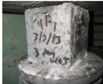
Fig. 5: Bulging failure mode of CPFRC specimens at peak load
