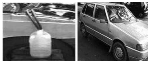
Fig. 1: External tank and of the fuelling lines of test vehicle
