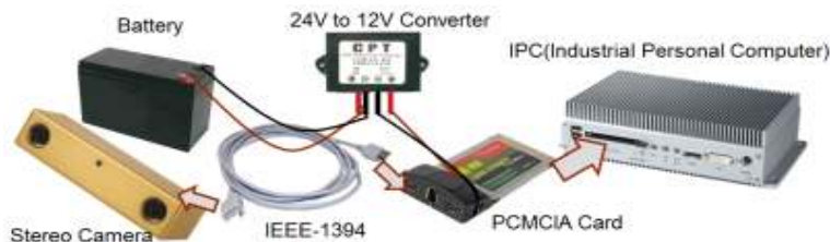
Fig. 3: The components of the stereo vision system
