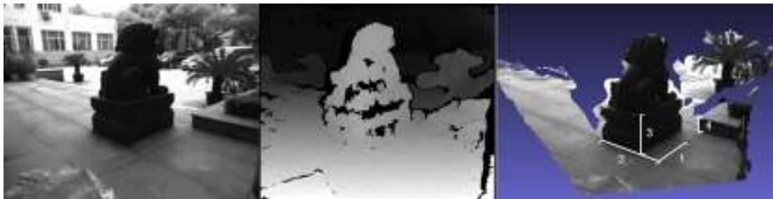
Fig. 4: From disparity image to 3D point cloud map
