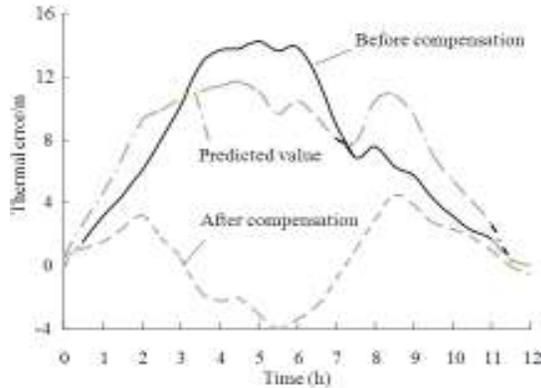
Fig. 8: The test results of the compensation system
