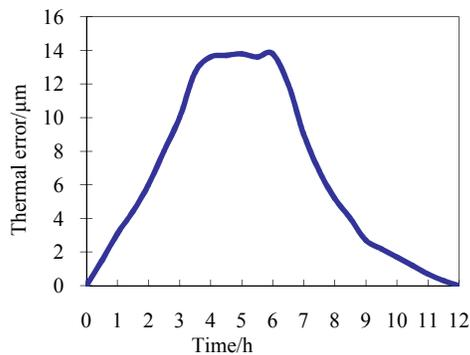
Fig. 4: Thermal errors of the spindle in the radial direction
