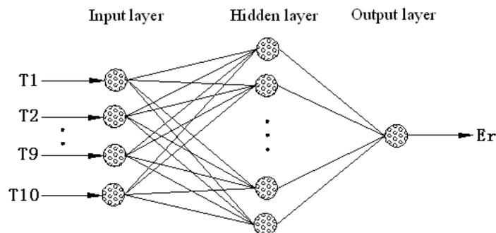
Fig. 5: The structure chart of BPN
