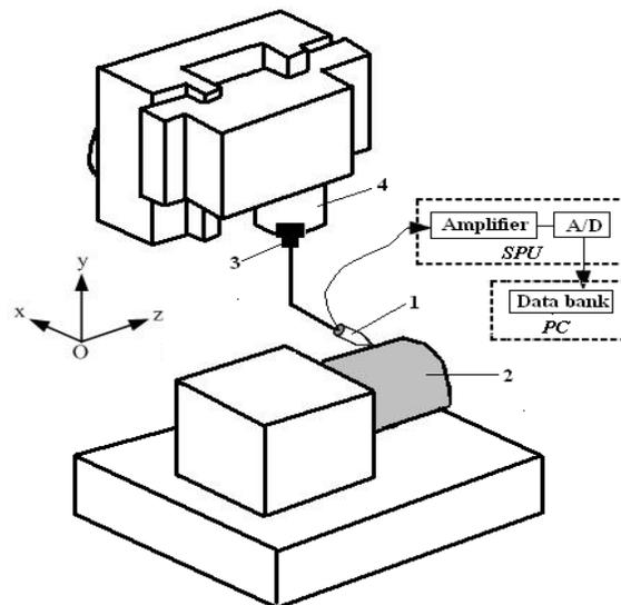
Fig. 2: The capacitance sensor mounted on the tool turret
