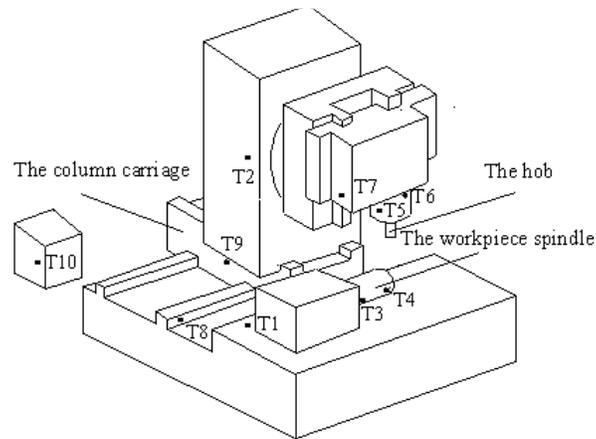
Fig. 1: The tested YK3610 hobbing machine
