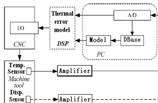
Fig. 7: Thermal error compensation system
