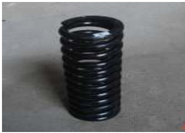
Fig. 3: Spring-settlement ( K = 100\text{kN/m} ) mm
