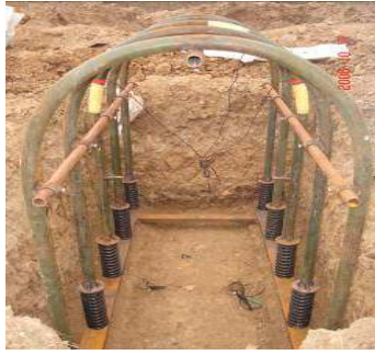
(a) Spring-settlement support structure
