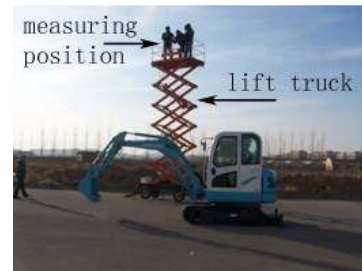
Fig. 4: Measurement of noise at hemispherical space measurement points
