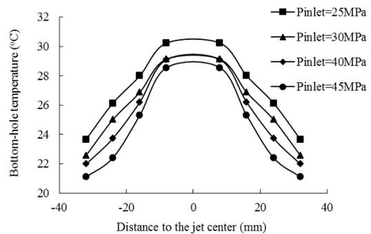
Fig. 6: Test of bottom-hole temperature
