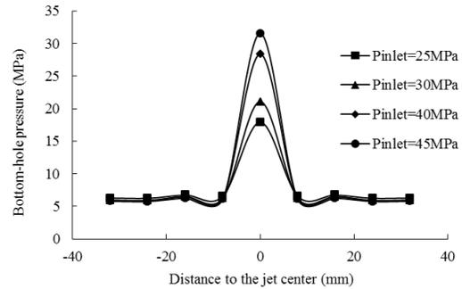
Fig. 5: Test of bottom-hole pressure
