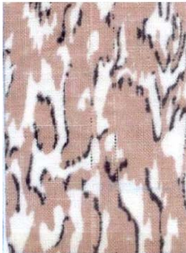
Fig. 4: Double warp (missing yarn)
