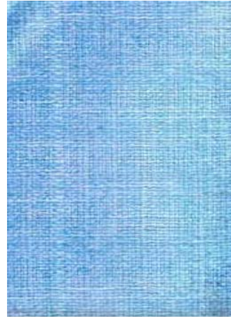
Fig. 5: Double warp (missing yarn)
