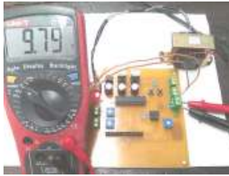
(a) Optocoupler testing,
