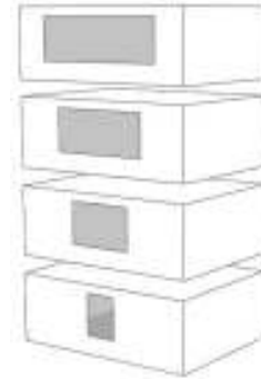
Fig. 2: Model 1 with various ratio window areas to floor area
