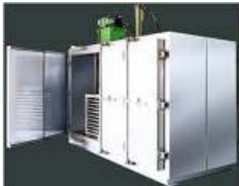
Fig. 4: The system of freeze DL-4, the temperature freezing environment (-50 ÷ -45) °C
