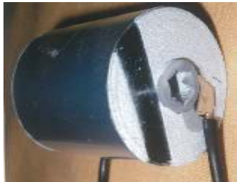
Fig. 5: Photo graph of sprayed end with partial edge disconnection
