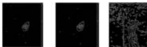
Fig. 2: Prewitt filter, sobel filter and canny filter
