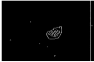
Fig. 4: Edges of the original image using sobel filter
