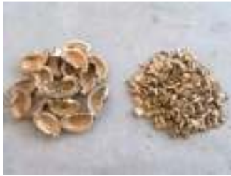
Fig. 2: Rubber seed shell (left side) and crushed rubber seed shell (right side)
