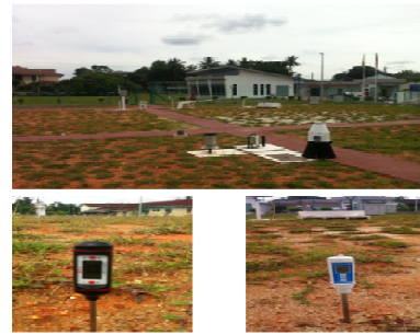
Fig. 2: Sample station sitiawan (upper) where Ts thermometer (left) and moisture probe (right) are placed
