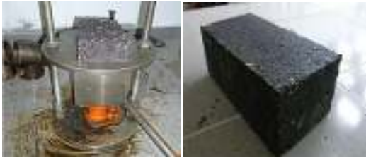
Fig. 5: Extruding of asphalt block from steel mold by jacking
