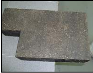
Fig. 8: The interconnections of asphalt blocks
