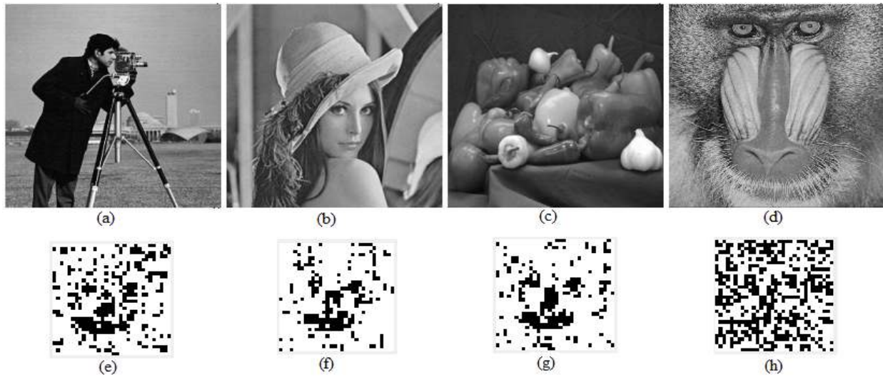
Fig. 18: Watermarked, (a) cameraman, (b) Lena, (c) peppers, (d) baboon images with 3 \times 3 median filtering and corresponding extracted watermarks (e-h)
