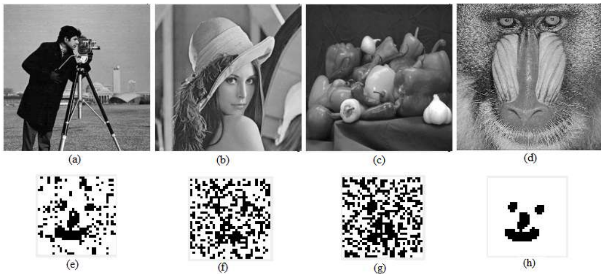
Fig. 17: Watermarked, (a) cameraman, (b) Lena, (c) peppers, (d) baboon images with 30% jpeg compression and corresponding extracted watermarks (e-h)
