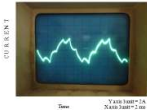
Fig. 23: Line current of inverter with IM-load
